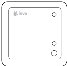
Single channel receiver for combi boilers
